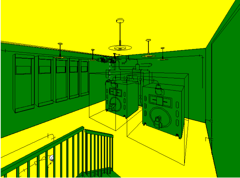
Figure 7. 3D Perspective view of Building A Boiler Room with Condition Index (CI) visual filter.
